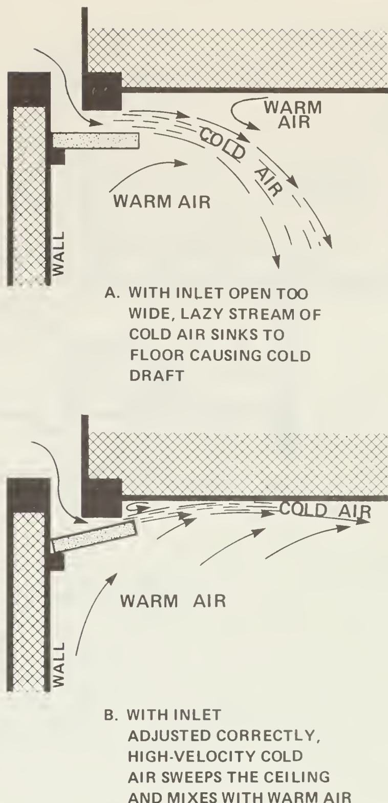
Figure 20 How the size of an air inlet slot affects the jet of cold air.
