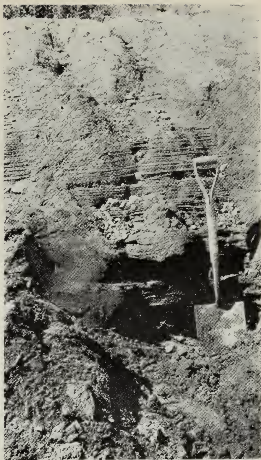
FIG. 3.—Road cut through the Riverbank Sandy Silty Loam. Recent rain has removed all the loose soil showing distinctly the alternate layers of silt and sand.
