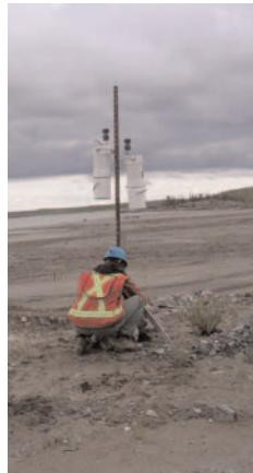
Worker checking an air monitor
