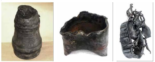
Because the failed components were so badly damaged, the teardown focused on the mate R3 bearing assembly, which likely had experienced a service life and usage similar to the failed bearing.
