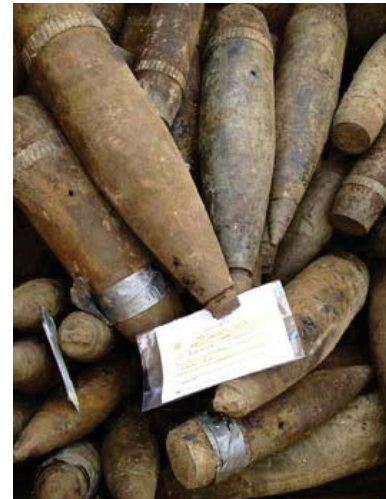
Projectiles dredged from Lac Saint-Pierre are perforated to prepare them for safe transport.
