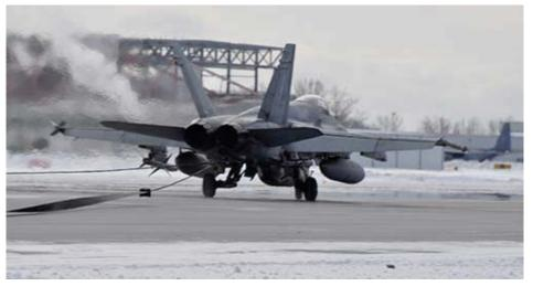
The cable passes this test as it hooks the CF-18 aircraft and brings it safely to a halt. *Photo by John Bruyea*
