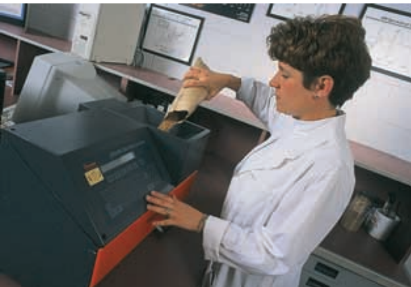
Jan Knight of the Canadian Grain Commission evaluates a grain sample in an NIR machine, an example of Automated Quality Testing already in place.
