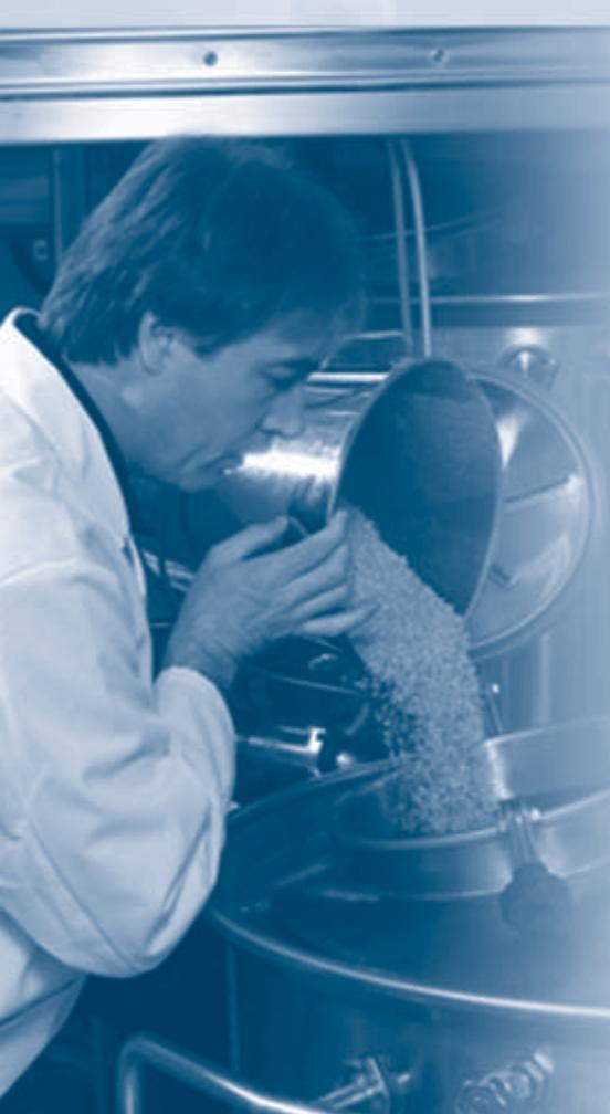
*Rob McCaig pours ground malt into the mash mixer, which converts starch into sugar. The CMBTC's malting and brewing facilities provide technical support to the grower, malting barley breeder, handling companies and traders, and maltsters and brewers.*
