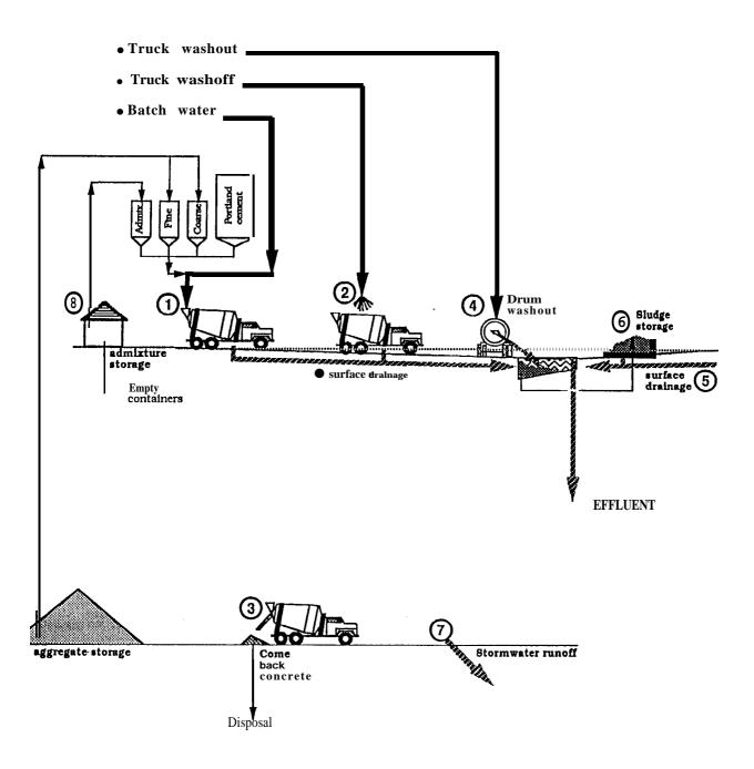
FIGURE 1: Typical components of batch ready mix concrete production
