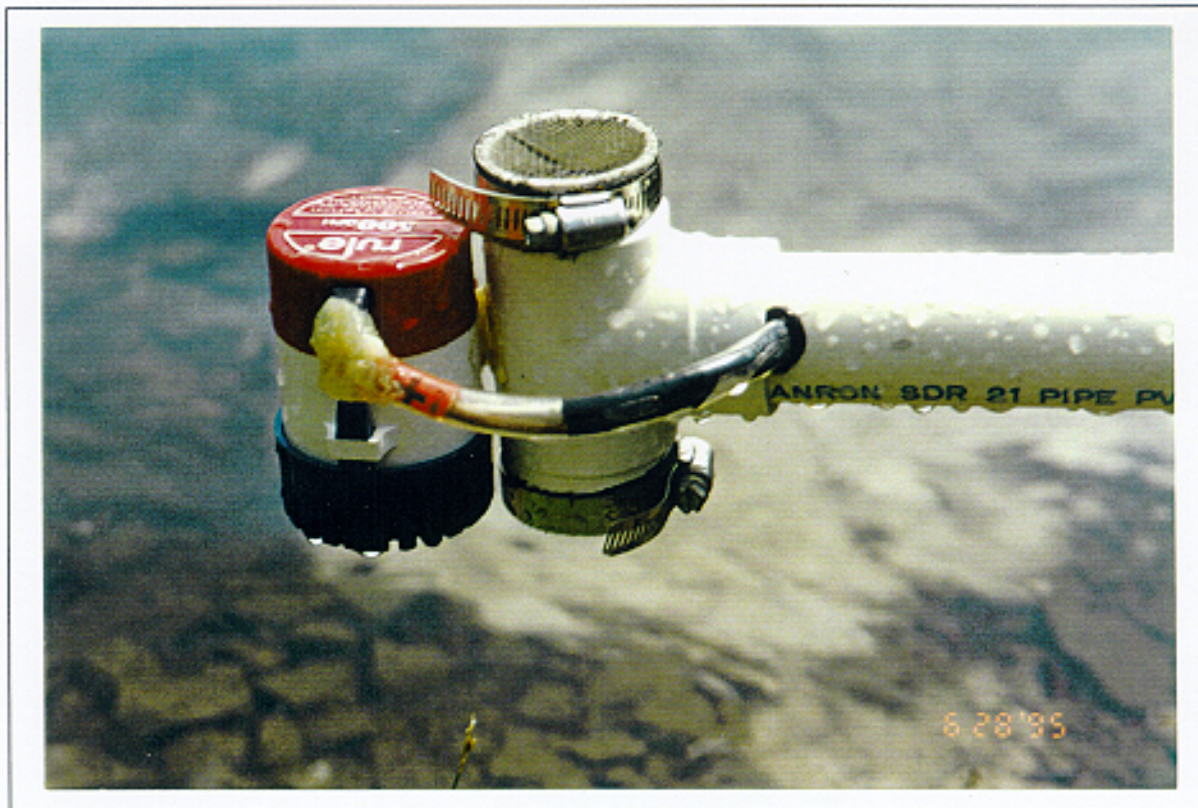
Plate 4. Water Intake Pump on Fluorometer Probe
