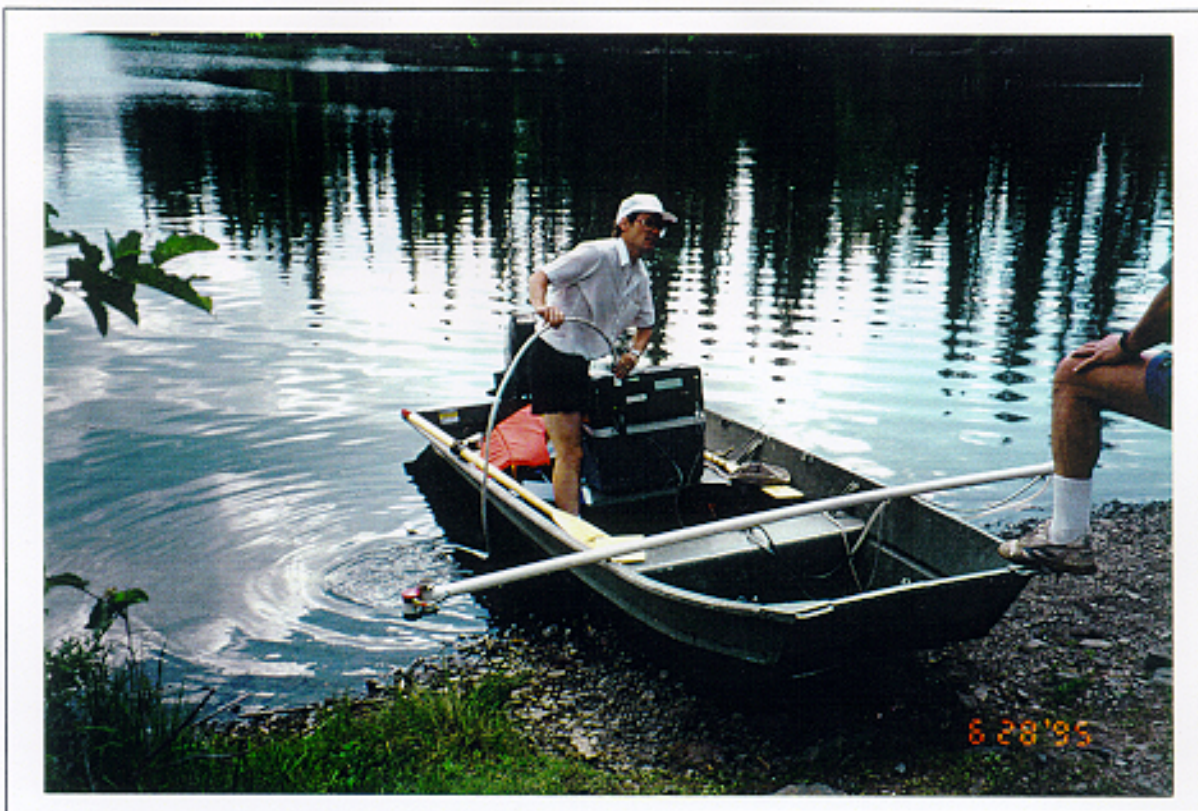
Plate 3. Fluorometer Configuration for Sampling from a Small Boat
