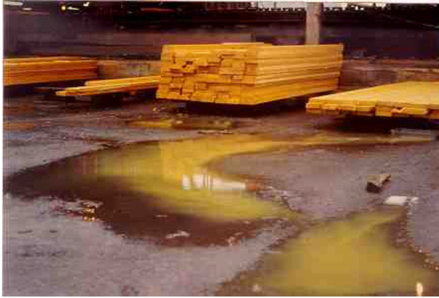
Photo #1: Leaching of Chlorophenates from Freshly Treated Lumber Prior to Implementation of Regulations. (3)
