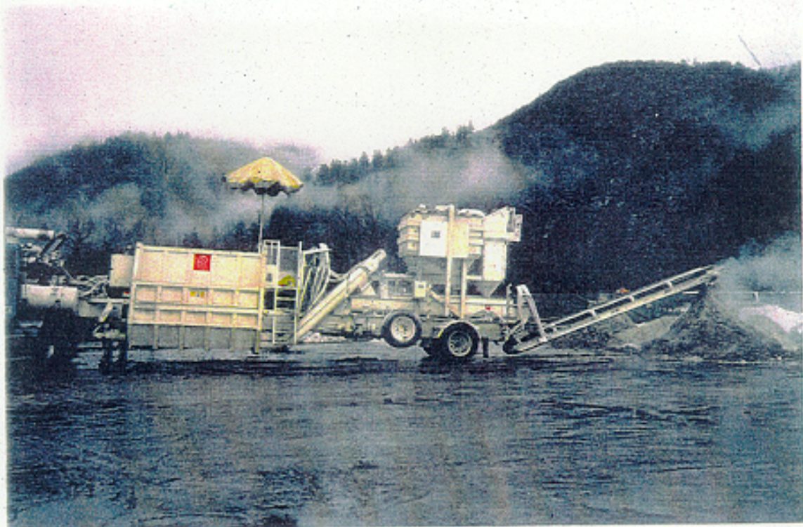
Fig. 1 CLC Mobile lime treatment plant, Agassiz, B.C.
