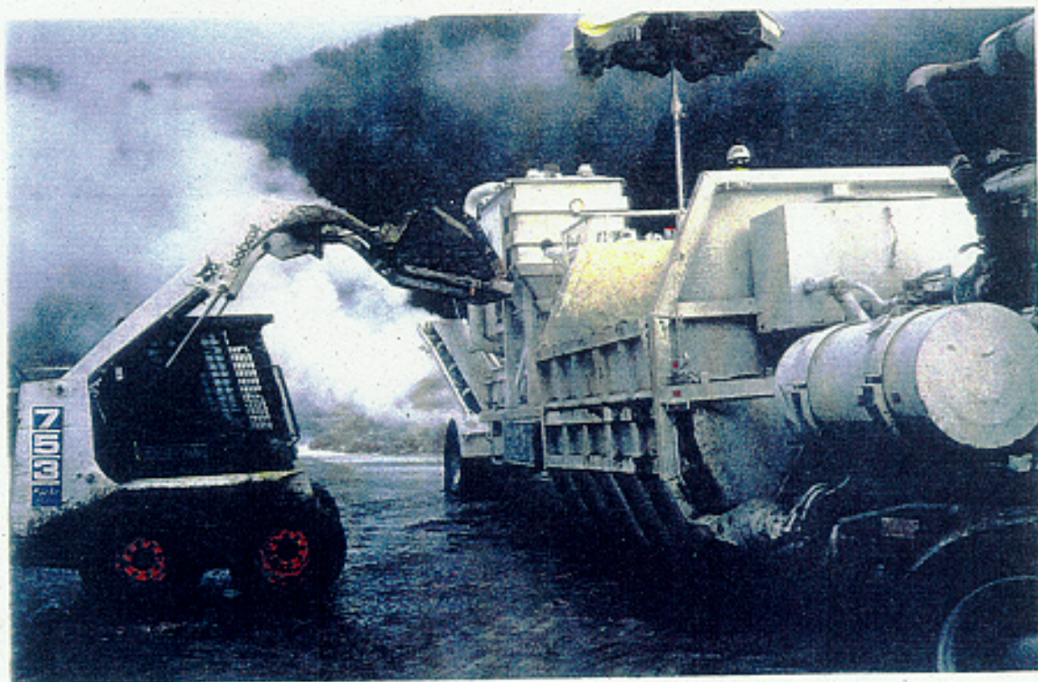
Fig. 2 Loading blending hopper with fish waste.
