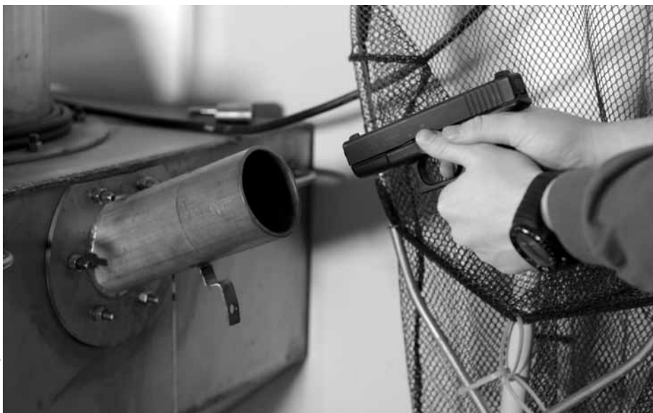
Projectiles fired into the tank lose their energy when they hit the water and sink to the bottom, where they can be retrieved and analyzed.
