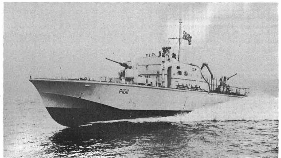
Powered by three gas turbines, HMS Brave Borderer , first of two Brave class fast patrol boats ordered by the Royal Navy, attained a speed of over 50 knots during trials in January. (Fifty knots equals about 57.5 land miles per hour.) A sister boat, Brave Swordsman , will be ready for service later this year. The craft can do duty either as motor torpedo boats or motor gunboats. (Photo from U.K. Information Office.)
