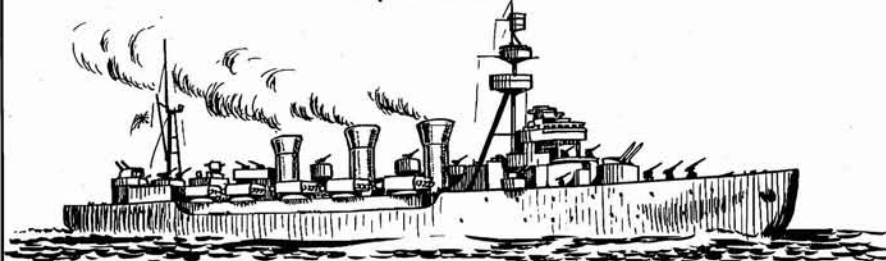
JAPANESE 'KUMA' CLASS CRUISERS, REFITTED AS 'TORPEDO CRUISERS' IN WORLD WAR II, CARRIED THE HEAVIEST TORPEDO ARMAMENTS AFOAT... FORTY 24-INCH TORPEDO TUBES.
