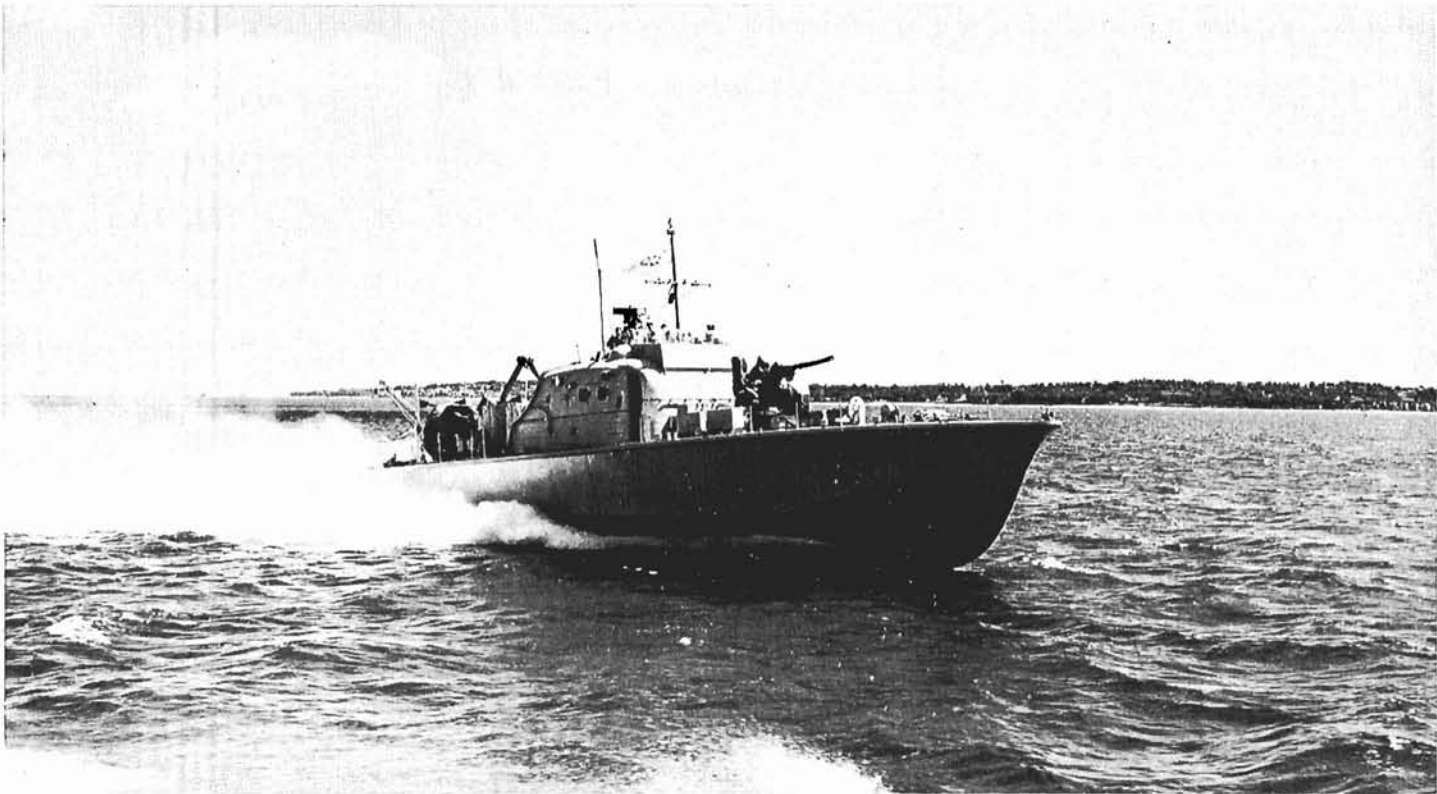
Is this, as her builders believe, the world's fastest warship? HMS Brave Borderer, first of a new class of fast patrol boats (convertible torpedo/gunboats), exceeded 50 knots on trials. Powered by three Marine Proteus gas turbine engines, developing 10,500 horsepower, she is of composite aluminum and mahogany construction. She and her sister ship, Brave Swordsman, were designed and built by Vosper, Limited, Portsmouth. (Photo from Bristol Siddeley)
