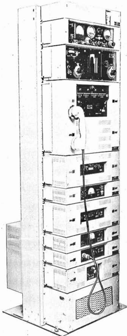
The Collins AN/URC 32 single sideband transceiver, which will be installed in Mackenzie class destroyer escorts. Communications equipment in these ships will be almost entirely located in a single communications control room. (O-14192)
