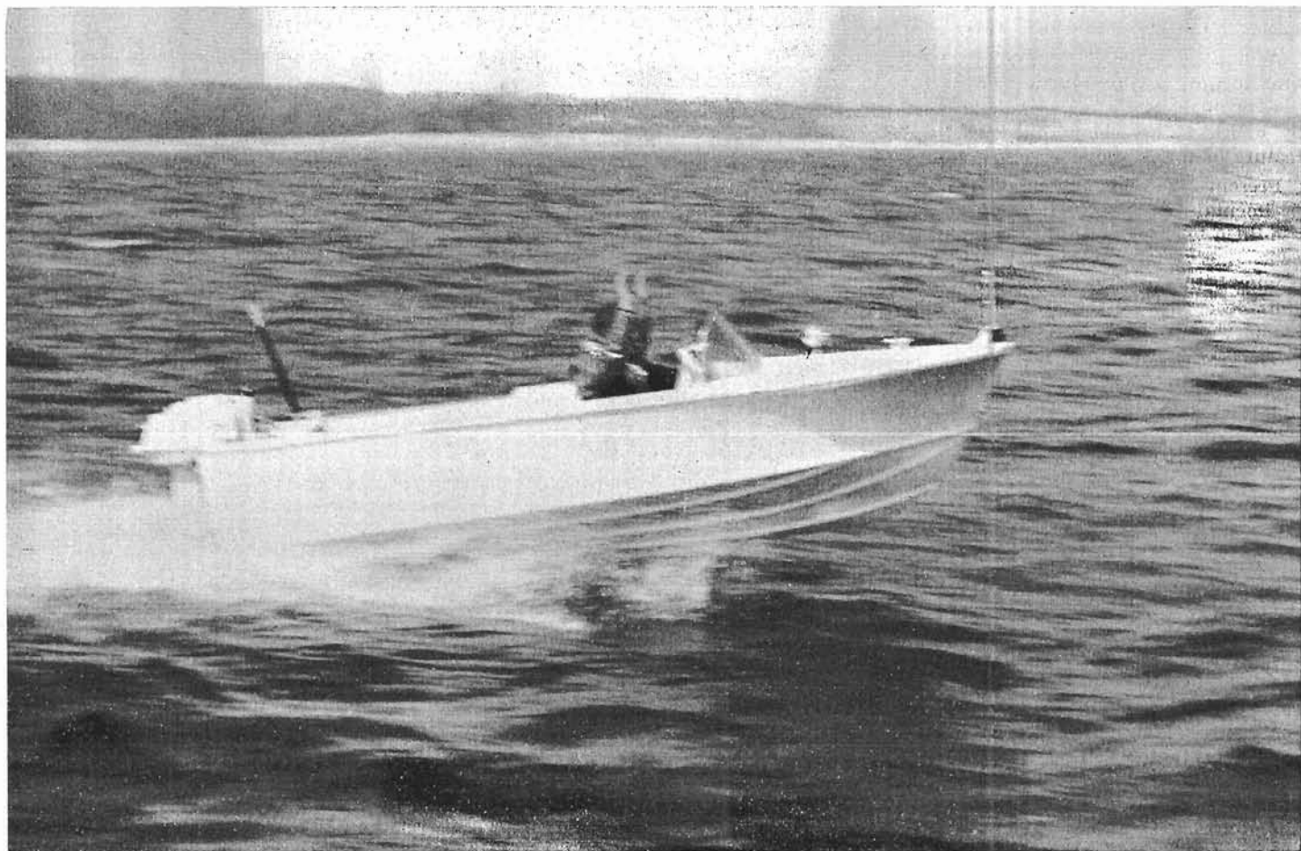
"Look, Mal No hands!" The Hunt 14-foot hydrolift hull is shown under test for the maintenance of longitudinal stability. (O-13816)
