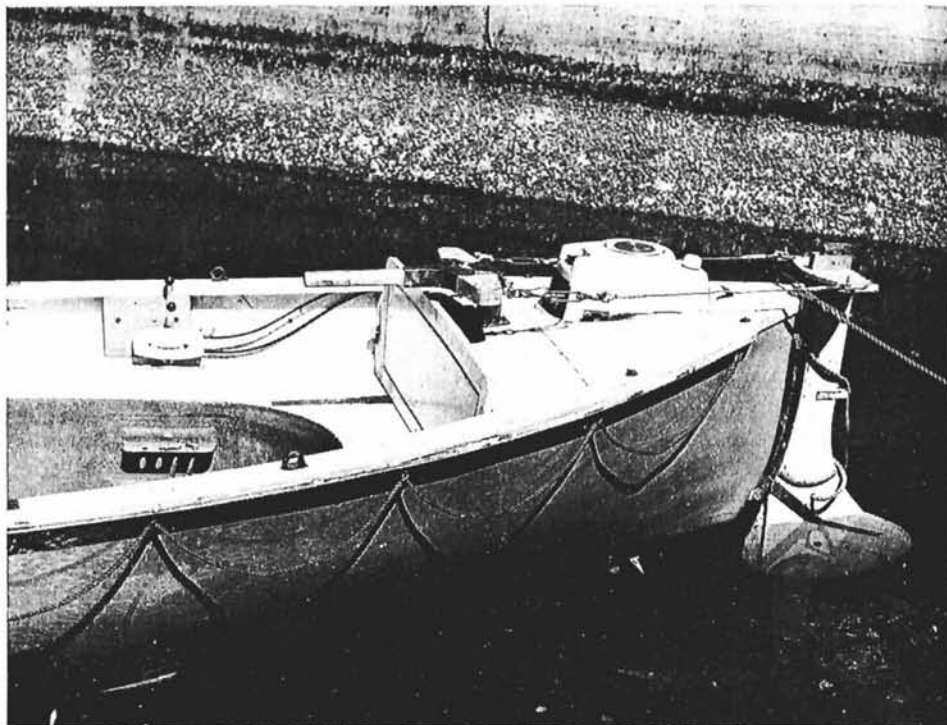
Eighteen horsepower outboard engine installed in a well in a 27-foot plastic whaler. The boat will exceed seven knots this power and motor installation does not affect sailing or pulling. (E-62083)
