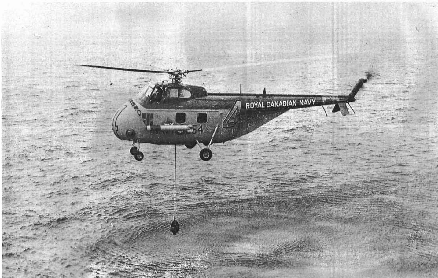
The helicopter is regarded as having many advantages as an anti-submarine weapon. It can outspeed any type of submarine, carry out a sonar search and attack with homing torpedoes. (DNS-24081)
