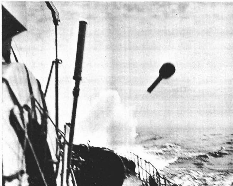
No lollypop, but a depth charge, with carrier or "flower pot" attached leaving the Y-gun of a Fairmile. (GM-0114)
