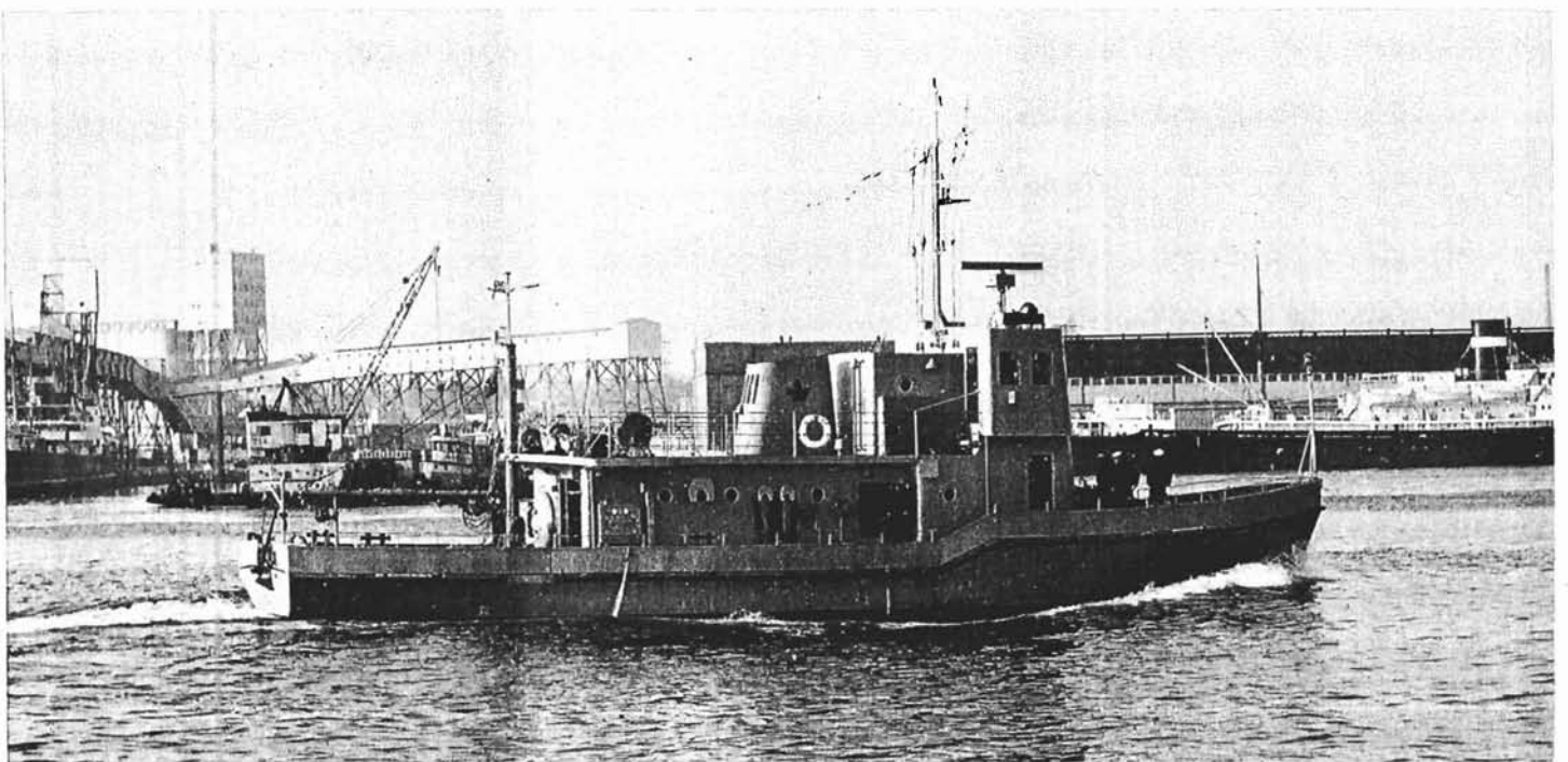
A custom-built diving vessel, YMT-11, was completed in January at Ferguson Industries, Pictou, N.S., for the Navy and began trials off Halifax. She is 88' by 20' by 4'9", with a speed of nearly 11 knots, can dive four men at a time to about 250 feet and is fitted with a recompression chamber. (HS-67277)
