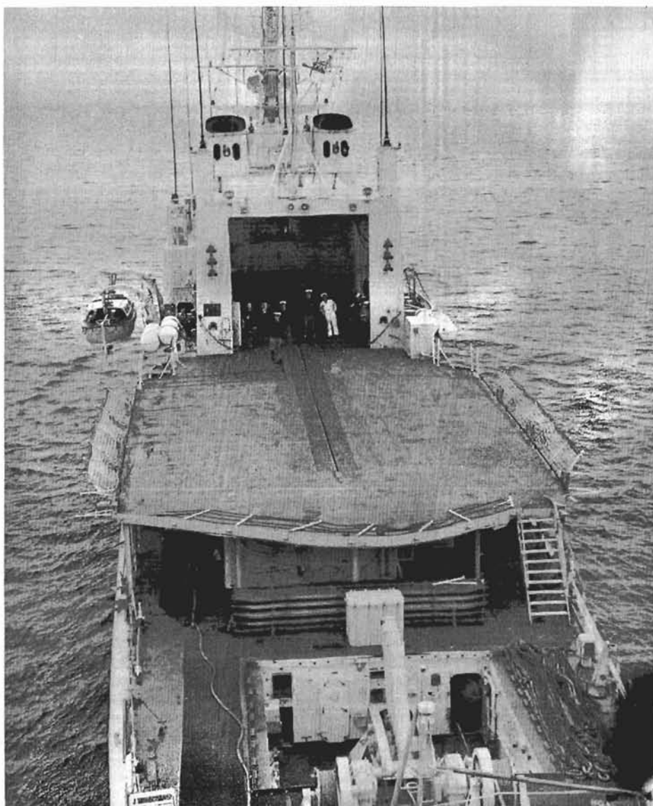
This is a 'copter-eye-view of the converted Assiniboine in which such new features as the variable depth sonar winch, triple-barrelled anti-submarine mortar (there used to be two sets of mortars) and the athwartship twin funnels can be seen. The slot in the flight deck is to accommodate the "Bear Trap" or down-haul winch, which will steady helicopters landing on a pitching deck. (E-73287)
