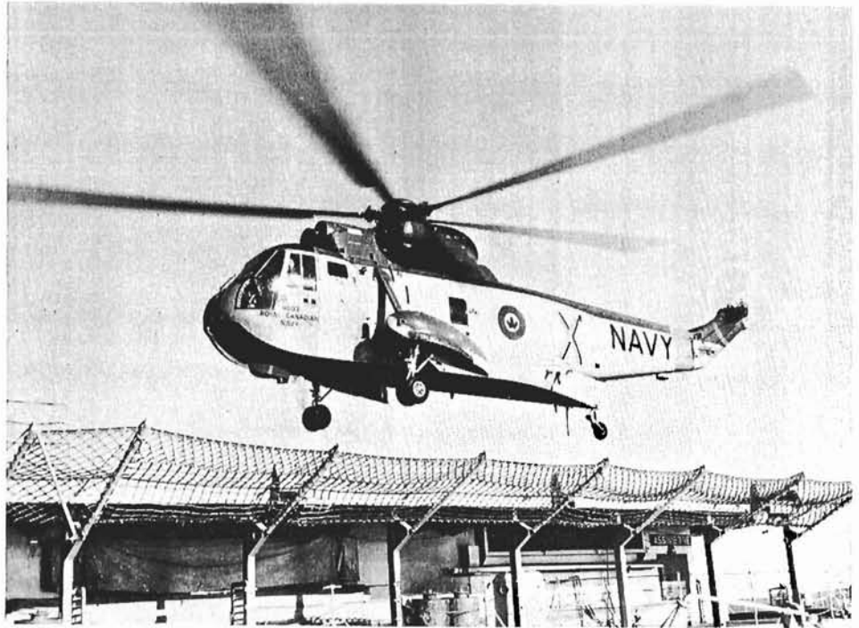
A Sea King, one of the big, swift, turbine-powered helicopters which will operate from the RCN's Annapolis class converted St. Laurent class destroyer escorts hovers over the flight deck of the Assiniboine . (CN-6759)
