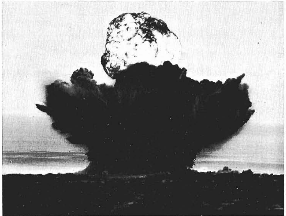
The Second Sailor Hat test charge is detonated on Kahoolawe island, Hawaii, to determine the blast effect on modern ships and weapon system. The 500-ton charge was detonated by the U.S. Navy at 3:21 pm, April 16, one of the ships exposed to the blast being HMCS Fraser . The Sailor Hat tests, conducted by the USN under the sponsorship of the Defence Atomic Support Agency, will end with the third and final detonation in mid-June. The first detonation occurred on Feb. 6, with the Fraser present on that occasion. (U.S. Navy Photo)
