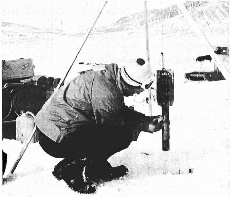
A bathythermograph slide is inserted before recording water temperature at varying depths. In the background is Vanhauven Pass, a valley which links Otto and Hare Fiords off Nansen Sound.
