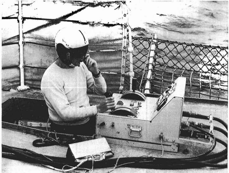
Amid multi-wired cables, the landing control officer prepares to haul down the tethered Sea King. The LCO is constantly in radio voice contact with the helicopter pilot. (CN-6826)
