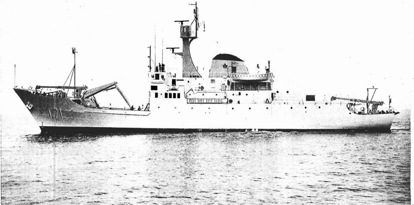
CNAV Endeavour, the first oceanographic survey ship to be built for the Department of National Defence, was accepted March 9 at Yarrows Limited, Victoria. The Endeavour is 236 feet long, displacing 1,560 tons, has a bulbous bow to reduce pitching, a transom stern and a fairly high rise of floor plate along with considerable flare above the load water line. She has roll reduction flume tanks and her two diesel electric motors can drive her 10,000 miles at 12 knots. She has a helicopter flight deck. Hitherto the defence department has used warships converted to the scientific role. (DRB Photo 4381-1)
