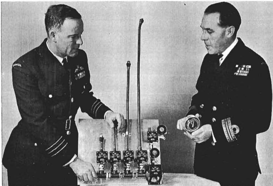
The co-inventors of the decompression computer are Wing Cdr. R. A. Stubbs and Surgeon Lt.-Cdr. D. J. Kidd, both of the Institute of Aviation Medicine, Toronto. The original "breadboard" model of the computer, assembled from parts of aircrew breathing equipment, is at the left. Surgeon Lt.-Cdr. Kidd is holding a prototype of an operational instrument.
