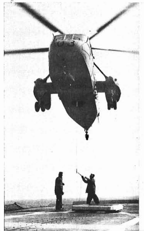
A flight deck crewman grounds the messenger while the other prepares to connect the haul-down cable. The Sea King hovers about 50 feet above the deck. (DNS-33897)
