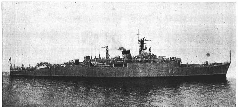
A former destroyer, HMS Relentless, is pictured leaving Portsmouth harbour for trials following her conversion to an anti-submarine frigate. The Relentless and her sister-ship, HMS Rocket, are prototypes embodying a number of new features. The conventional bridge has been taken away and in action the captain would "fight" the ship from an operations room, a periscope giving him an all-round view. The destroyer escorts being built for the RCN will have a similar arrangement. (UK Information Office photo).
