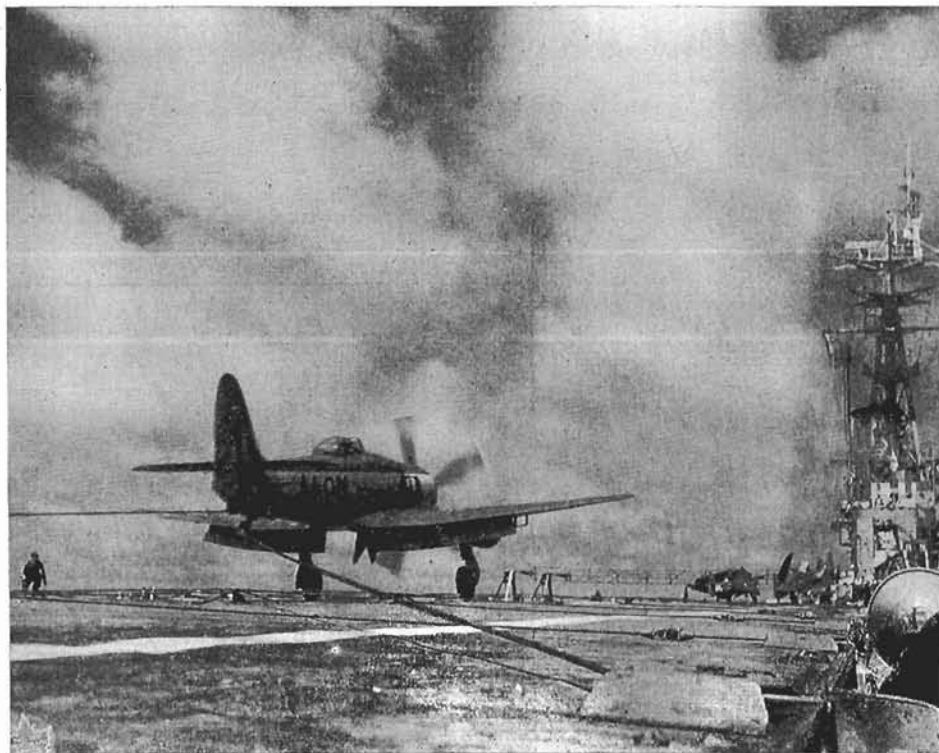
A Sea Fury of 871 Squadron catches an arrester wire in landing on the flight deck of the Magnificent during flying exercises in which the aircraft of 30 Carrier Air group spent 1,016 hours in the air in the month of August — a new record in the RCN. (MAG-3256).
