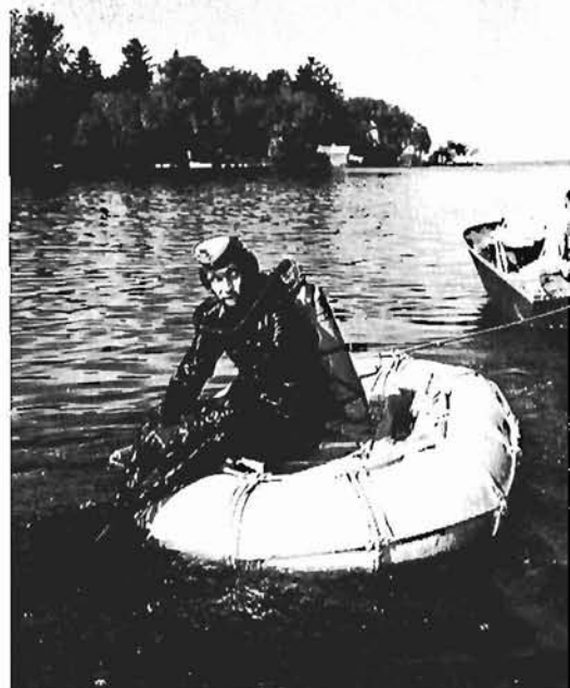
Ord. Lt.-Cdr. G. D. Cook tests the sea-worthiness of a new fibreglas Carley float built in HMC Dockyard, Esquimalt. The float is rot-proof and unsinkable. (O-6005)
