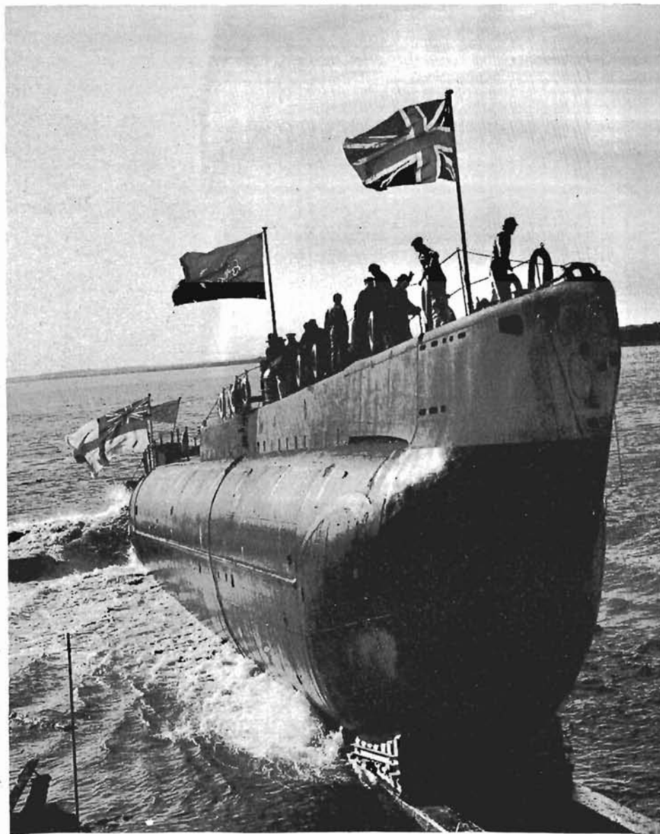
Gliding down the slipway into the water after her launch recently is the Explorer, a new experimental submarine for Britain's Royal Navy. An outstanding feature of the hydrogen peroxide powered vessel is that she can remain submerged for long periods without the use of a "Snort" breathing apparatus. She has a high underwater speed. (Admiralty Photo)
