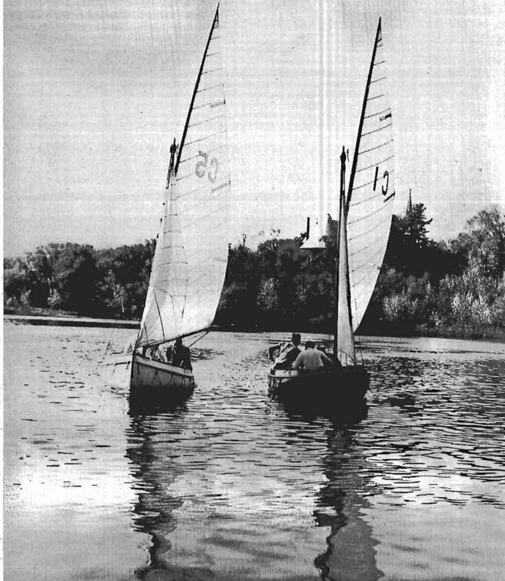
Crews compare the performances of two dinghies under sail. On the left is a prototype 14-foot dinghy built of polyester resin reinforced with fiberglas cloth and mats. It is the first boat of this type of construction to be built for the RCN. (O-6014)
