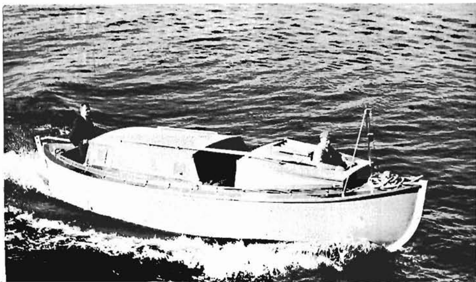
The 27-foot Canadian motor sea boat is shown going through its paces at the Arnprior "regatta". This boat is a modification of the Royal Navy motor sea boat, the main difference being a whaler stern, greater power and omission of the mast and sails. (O-6008)
