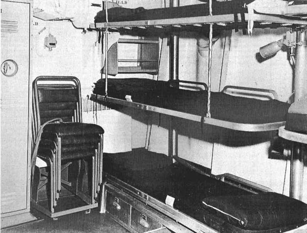
This shows a corner of a Chief and POs' mess. The middle bunk can be lowered to form the back for a settee. Bunks are equipped with individual reading lamps and foam mattresses. Gear is stowed in drawers below bottom bunk and in individual lockers, of which one is shown at the left. Nesting chairs provide additional seating. (ML-1510)
