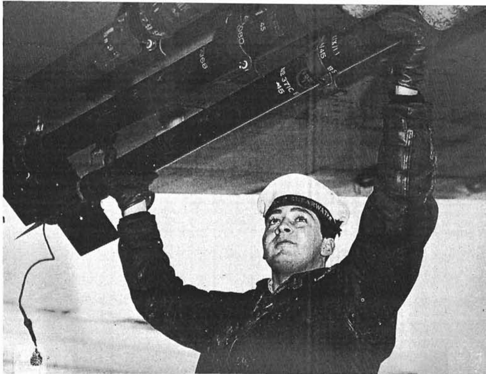
Attaching a practice rocket projectile to the wing of an anti-submarine Avenger aircraft in preparation for an aircraft armament demonstration is AB Robert Brown of Blenheim, Ont. This demonstration recently took place off the east coast of Nova Scotia. The aircraft taking part were from Shearwater . (DNS-13332)
