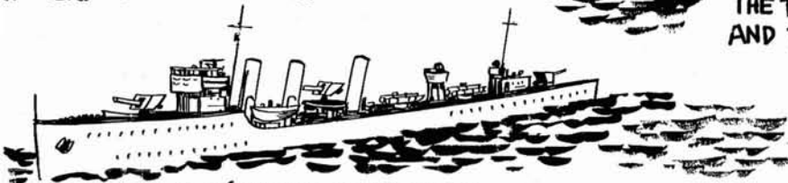
'L, M, N, R, & S' CLASS DESTROYERS OF WORLD WAR I - 3 4 IN. GUNS, 4 TORPEDO TUBES, 29-36 KNOTS...
