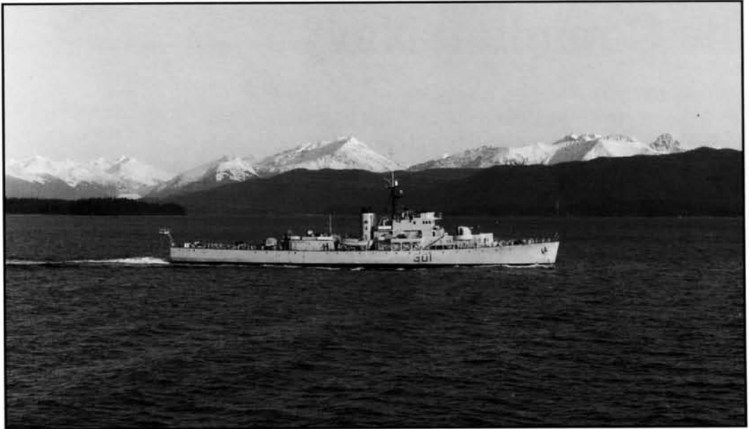
In addition to their Cold War anti-submarine patrols, the frigates deployed on extensive training cruises. The large deckhouse abaft the boat position visible here on HMCS Antigonish contained classroom and messing facilities for officer cadets under training. (Canadian Forces photo E-79010)
