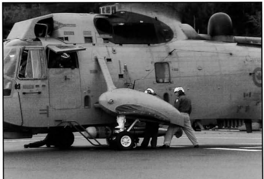
HS 443 Squadron personnel load a Mk-46 exercise torpedo at CFMETR in November 1999. (Photo: Cpl Mike Weber)
