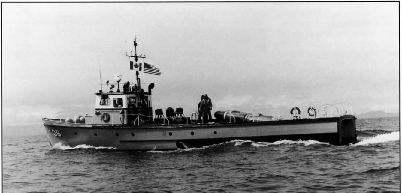
A United States Navy torpedo retriever boat stationed at CFMETR carries Canadian Mk-48 torpedoes being tested on the ranges. (Photo: Terry Berkley)
