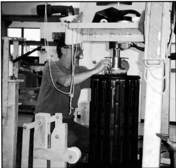
Sonar technician Bill Reynolds prepares a helicopter sonar hydrophone for in-water testing as part of the R&O process. (Photo: Terry Berkley)
