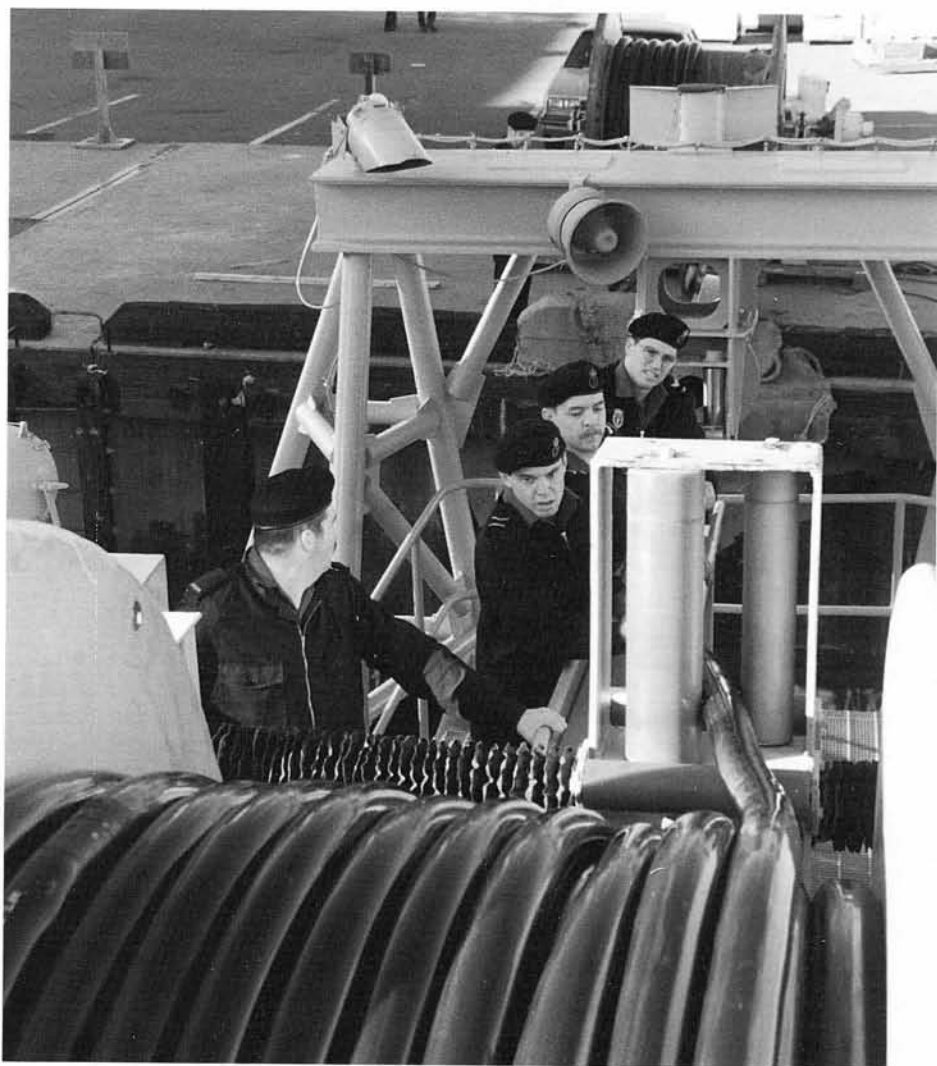
Naval Weapons Technicians land HMCS Fraser's towed array in Dockyard Halifax. The cable can be seen passing from the winch drum, aft through the horizontal and upright rolling fairleads of the level-winder, and out the stern of the ship through a bell fairlead.
