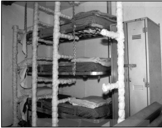
Fig. 2. This 2.5-metre x 3-metre concrete, steel-lined chamber was set up at the National Research Council facility in Ottawa in the late 1980s to conduct full-scale fire-testing of various shipboard furnishing materials. The chamber was outfitted with a typical three-bunk tier, settee and locker. As is explained in the text and illustrated in Fig. 3 below, the difference between the fire performance of old- and new-type furnishing materials was glaringly obvious.
