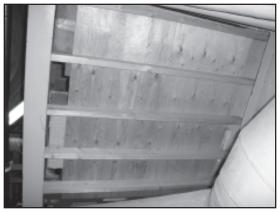
Fig. 2. Wooden storage platform located in a *Halifax*-class forward engine-room casing.
