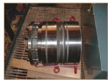
Step 7. The replacement clutch with its transport brackets installed.
