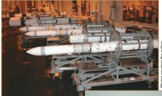
The RIM-162 Evolved SeaSparrow Missile carried on board the *Halifax*-class frigates offers much greater defensive capability than the RIM-7 missile it has replaced. A modified guidance section includes a quick-start feature for
