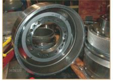
Step 11. The input assembly (shown here removed from the main sliding assembly) also showed no defects.
