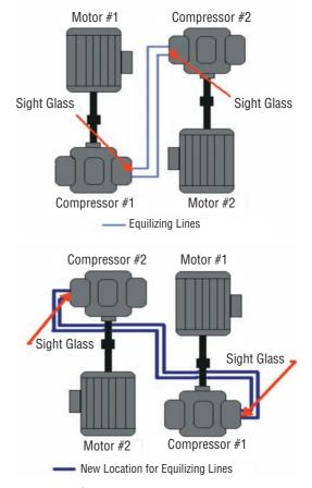
Figure 4. Compressor-motor assemblies before and after reconfiguration
