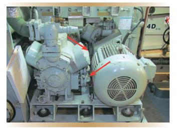
Figure 1. The refrigeration compressor configuration on board the *Halifax*-class frigates. The location of the two oil-monitoring sight glasses is indicated by the arrows.
