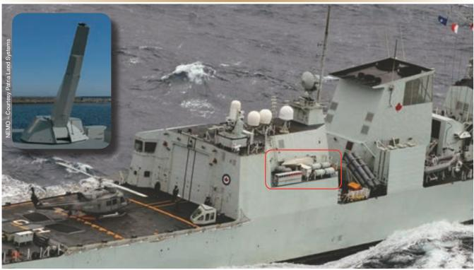
The author's proposed site for a precision-guided weapon mount on board some *Halifax*-class frigates is on the starboard mezzanine deck between the hangar and the funnel.
