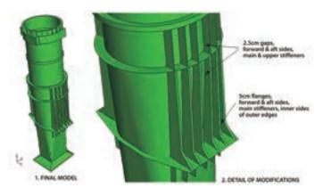
Figure 3. Model of the final uptake design with detail.
