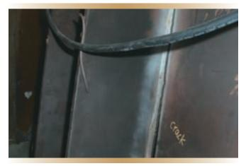
Figure 1b. One word says it all. Fatigue failure is the result when the shell of the intake is subjected to thermal expansion, but is constrained by the external stiffener.
