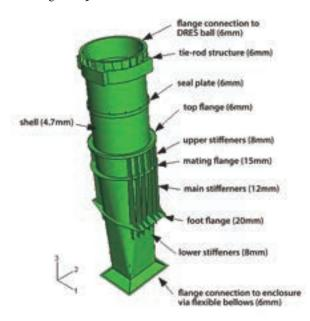
Figure 2. Original design of the original (existing) uptake with boundary conditions.
