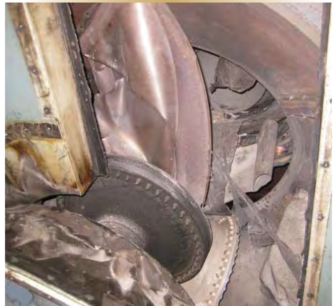
Figure 5 – What the exhaust duct (no. 1) and HSCS (no. 48) were supposed to look like – and what Toronto's engineering staff found.
