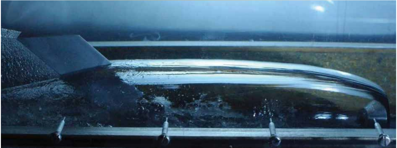
Figure 3 – Controlling a supercavitating body is a complex dance between aerodynamics within the gas cavity and hydrodynamics in the sea surrounding the bubble. (Source: http://cav.safl.umn.edu/gallery.htm )
