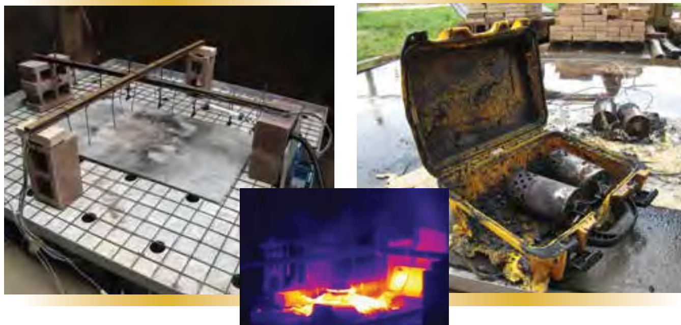
Figure 5 – To test an accidental discharge of the aerosol extinguishers inside the manufacturer supplied storage cases, instrumented cases fitted with thermocouples were set under a custom test rig to measure the radius of heat after a unit was activated. For both the DSPA and the StatX unit (inset photos), the cases held together well despite internal temperatures reaching 800°C.
