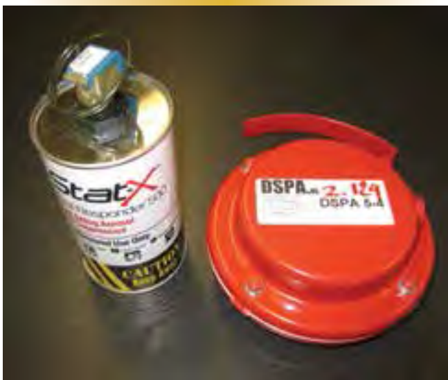
Figure 1 – Full-scale live fire testing was conducted at the University of Waterloo’s Fire Research Lab on these two variants of hand-activated aerosol extinguishers: the StatX First Responder ® (left) and the DSPA Manual Firefighter ® .
