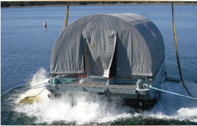
Figure 4. The floating platform carrying the MHP crane and support fixture reacts to a test shot from the submerged airgun array.
