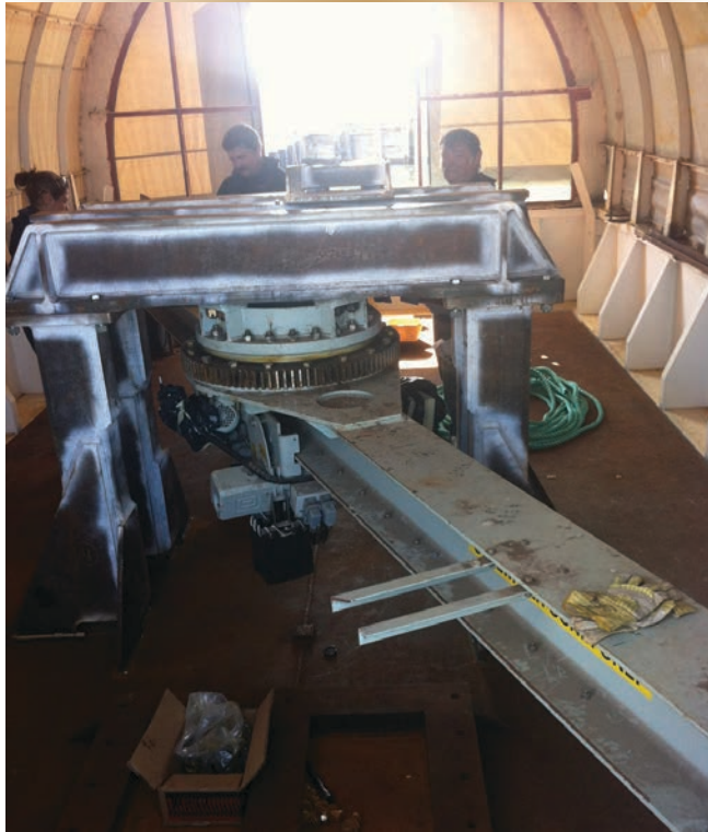
Figure 2. The MHP crane was coupled to a specially fabricated test fixture that was attached to an instrumented deck before being installed aboard NETE's floating shock test platform.
