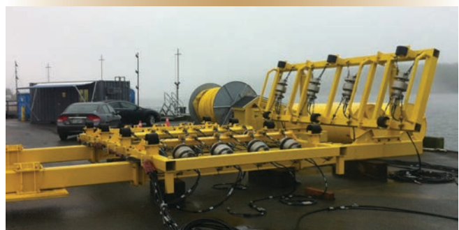
Figure 3. The airgun array assembly staged on the jetty at Shearwater at the south end of Halifax Harbour. While the use of airgun technology in lieu of traditional explosives was a first for DND on a commissioned heavyweight shock test equipment trial, the technology itself had been trialled in 2009 using a retired submarine as a test subject.
