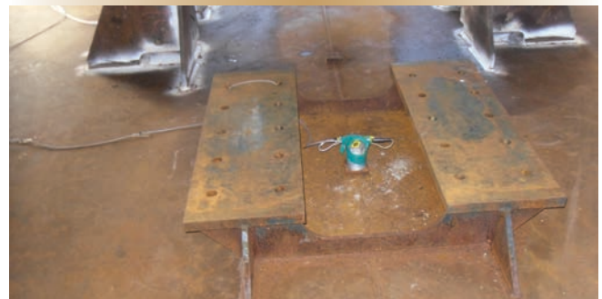
Figure 5. Accelerometers attached to the crane support (left) and to the heavy steel platform of the DSF II deck simulator fixture returned data that verified the proper execution of the heavyweight shock test trials, which were deemed a success.
