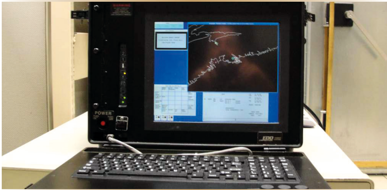
A stand-alone, ruggedized, portable link display system (PLDS) workstation and HF radio subsystem.
