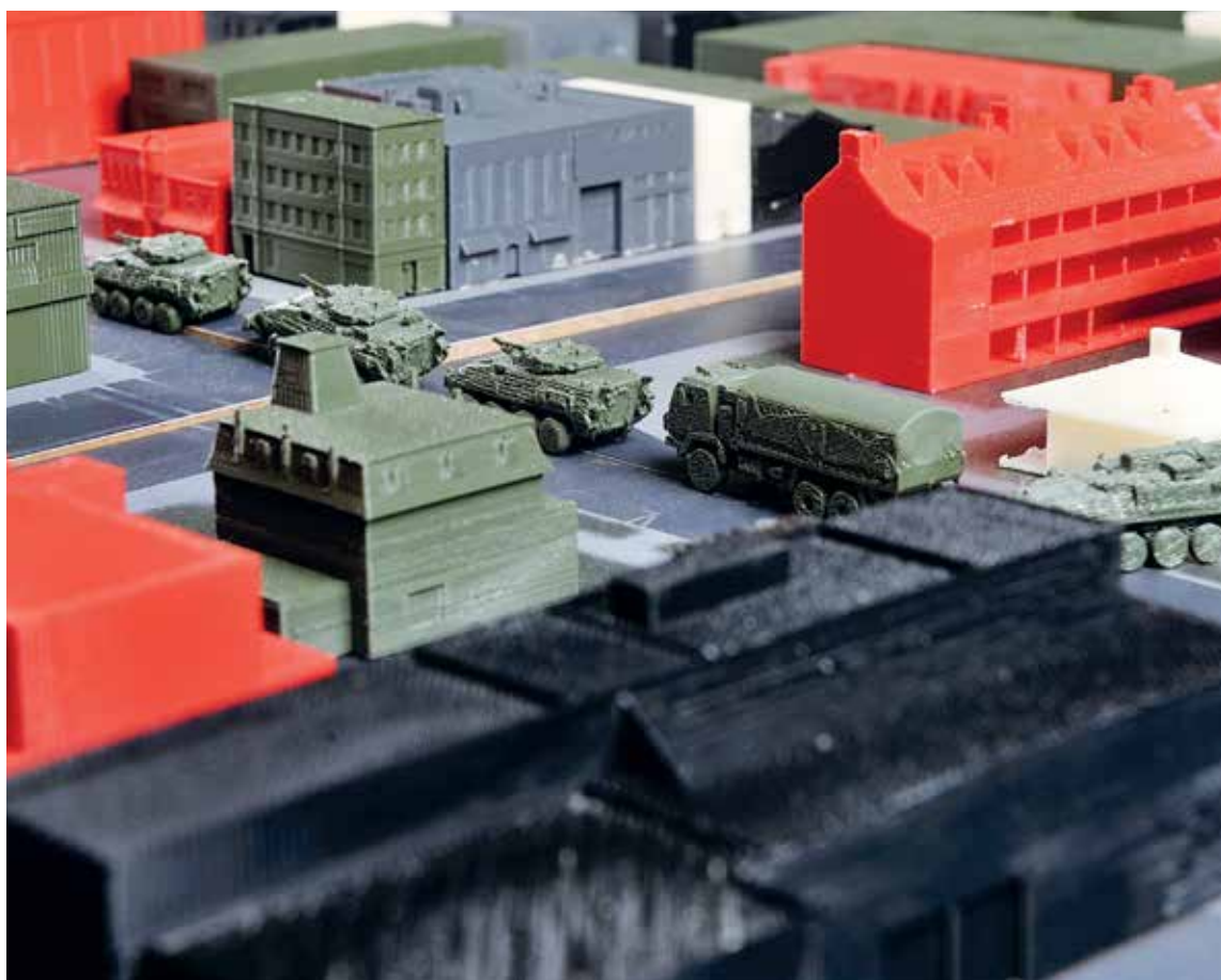
This two-metre by three-metre scale model of a 12 city block section of downtown Fredericton, N.B. was created using satellite imagery and 3D modeling software. All pieces, including the convoy of vehicles, were printed using 3D printers at the Army Learning Support Centre, 5th Division Support Group Gagetown.
