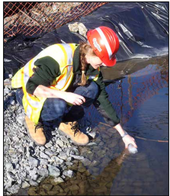
Monica Woods samples a sediment detention pond at a work site in northeast Coquitlam. Photo: Kelly Prystupa.
