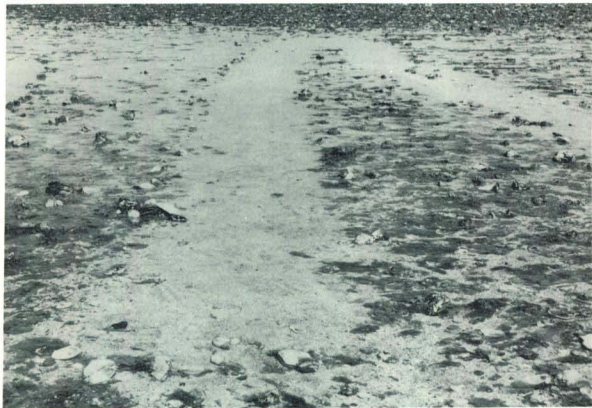
Fig. 8. Condition of plot dug by hydraulic clam rake after the plot has been covered for one tide.
