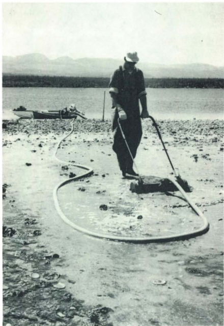
Fig. 5. Hydraulic clam rake in operation on dry flat at Seal Island, July 1966.
