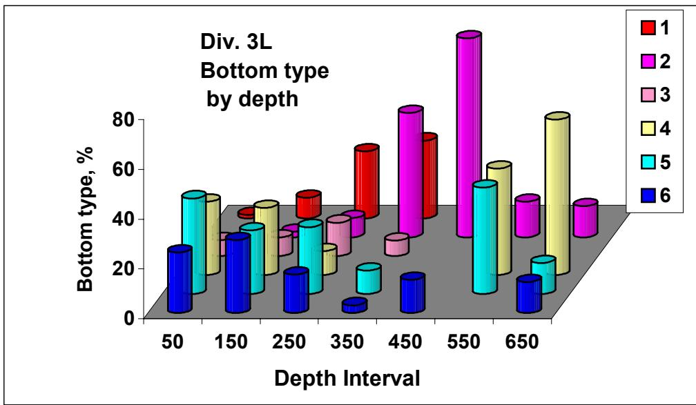
Fig. 6. Distribution of substrate type by depth from RoxAnn Seabed Classification System data for offshore Div. 3L (northern Grand Bank); bottom types range from dark red (softest and smoothest; in back) to dark blue (hardest and roughest; in front).
