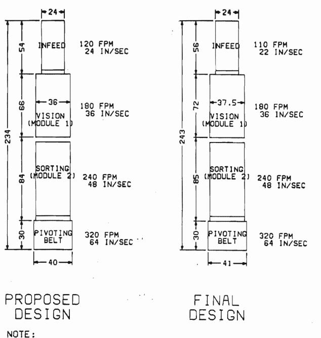
WIDTH DIMENSIONS ARE BELT WIDTHS IN INCHES. LENGTH DIMENSIONS ARE MACHINE LENGTHS IN INCHES.
