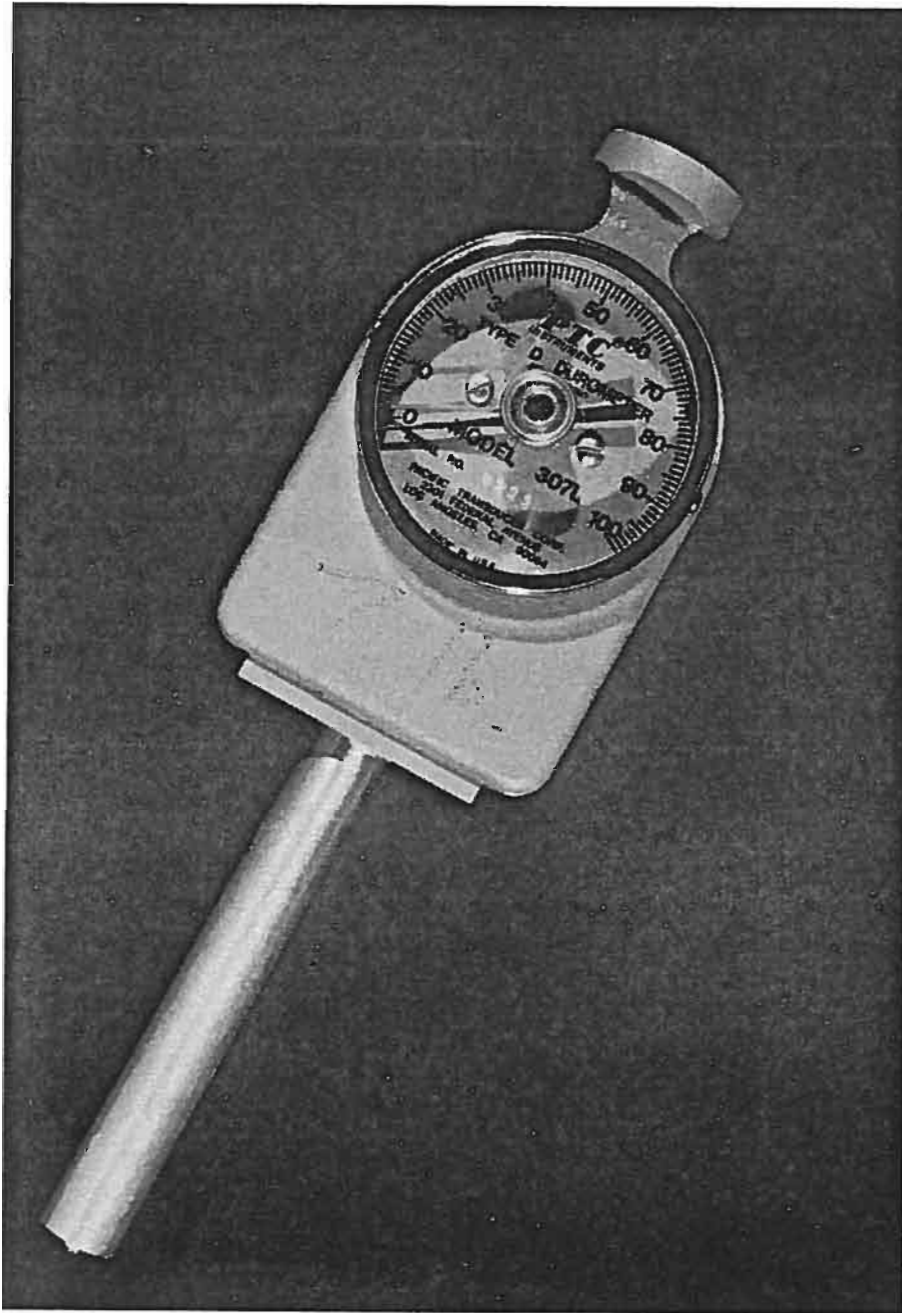
FIGURE 1. One of the modified Pacific Transducer durometers used in the study. The ancillary pointer (lazy hand), resting on 2 on the dial, is difficult to see in the photograph.
