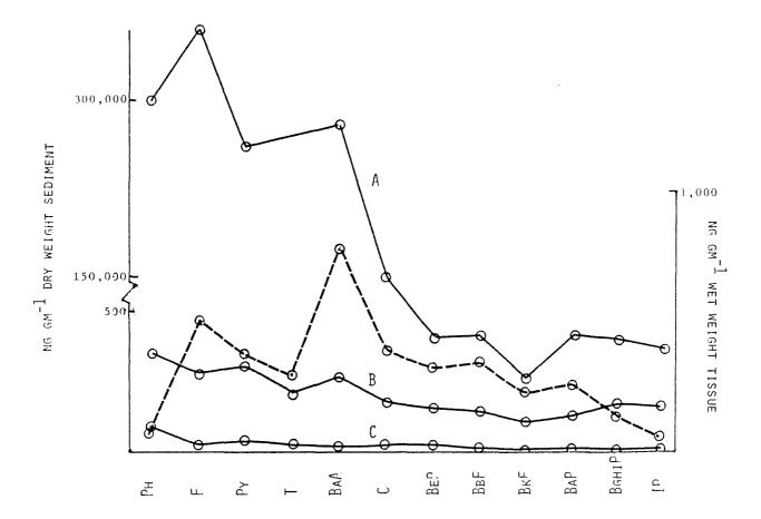
Figure 7. PAH composition profiles in contaminated bottom sediments from three Sydney Harbor locations (A - Muggah Creek, B - South Arm, C - North Arm) and bivalve mussel (dashed line). (Data from Matheson al. 1983).
