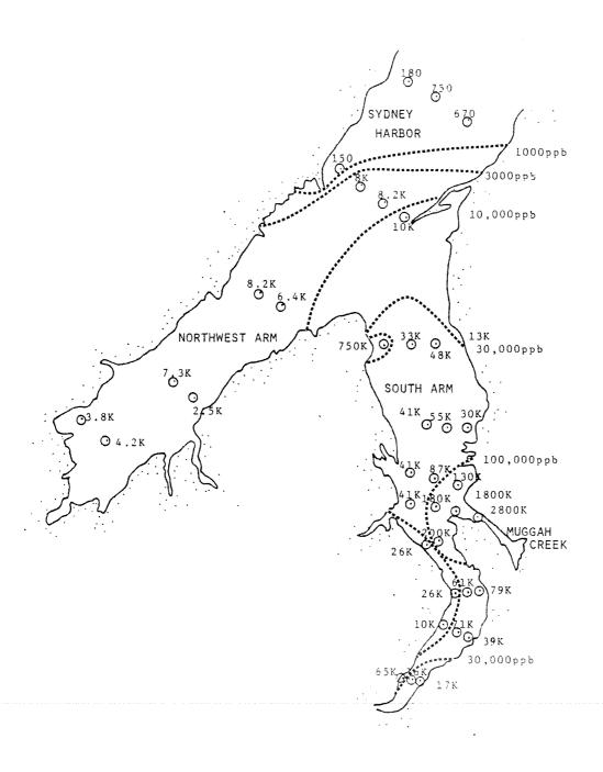
Figure 6. PAH concentration contours in bottom sediments from Sydney Harbor (redrawn from Matheson et al. 1983)
