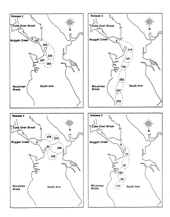
Figure 1. Flow patterns of dye (rhodamine w.t.) released at different times from Muggah Creek and Coke Oven Brook. (From Matheson et al., 1983)
