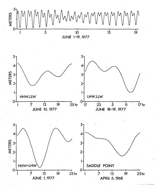
Fig. 2. Sequences of Tidal Extremes at Point Atkinson.
