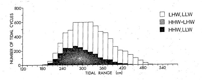
Fig. 3. 19 Years of Point Atkinson Extremes by Tidal Range.
