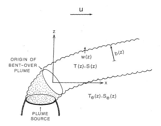
Figure 2. Schematic diagram of plume rise in an ocean crossflow of velocity U with environmental values of temperature  $T_e(z)$  and salinity  $S_e(z)$ . The origin for the plume calculations is at z=0. The stippled region between the real source and the origin is not explicitly modelled but the relation between source and origin values is given by (3.10).
