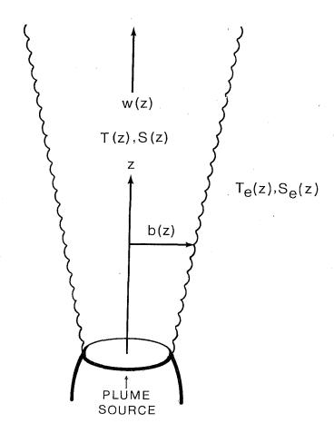
Figure 1. Schematic diagram of plume rise in a still ocean environment with environmental values of temperature  $T_e(z)$  and salinity  $S_e(z)$ .
