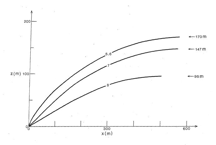
Figure 4. Plume trajectories for examples 5-8 of Table 1. Each trajectory is identified by its example number and its maximum height of rise.
