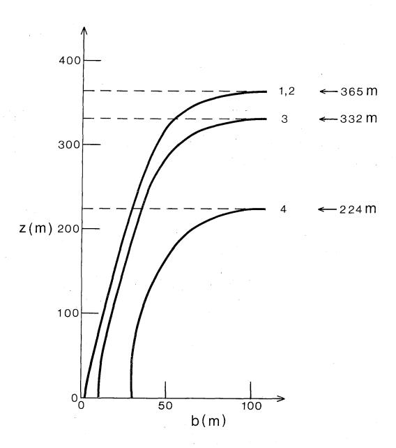
Figure 3. Plume profiles for examples 1-4 of Table 1. Each profile is identified by its example number and its maximum height of rise.
