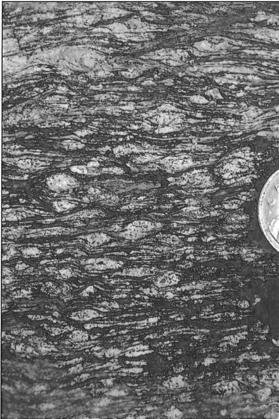
Figure 75. Strongly foliated gabbro/diorite with relict plagioclase crystals, Bohica mafic complex, Kaskawan Lake. Looking down on horizontal surface. The fabric could be termed protomylonitic. Note the sinistral shear bands. Coin for scale 2.5 cm in diameter. GSC 1994-170
