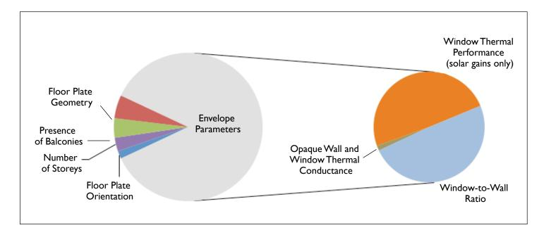
Figure 4 Relative Impact of Architectural Features on Cooling Loads
