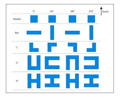
Figure I Building Floor Plates and Orientations Investigated
