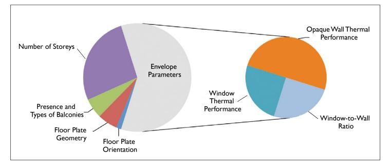
Figure 3 Relative Impact of Architectural Features on Heating Loads
