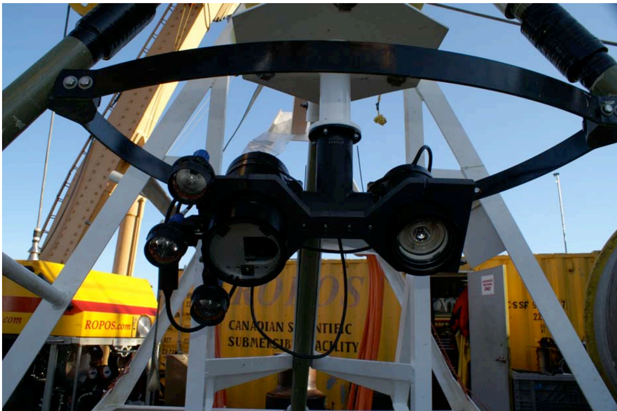
Figure 6. Close-up of underwater camera, "cyclops" and lighting array, before deployment
