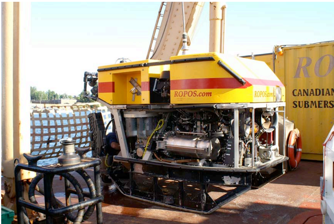
Figure 4. ROPOS, the remote operated vehicle used to deploy VENUS equipment and the carcass
