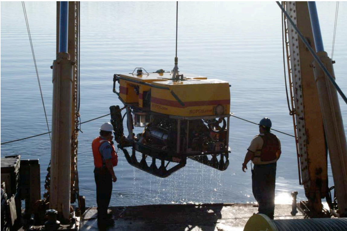
Figure 16. ROPOS being recovered after deploying carcass
