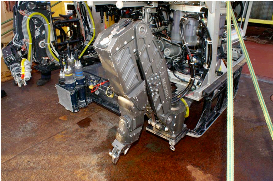
Figure 15. Raptor arm of ROPOS used to minutely position carcass under camera tripod.
