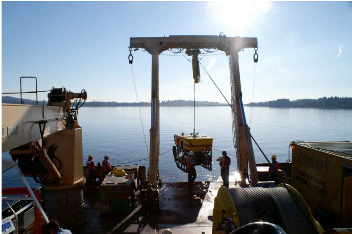
Figure 12. Deploying ROPOS prior to dropping pig carcass, for ROPOS to place carcass at camera site.
