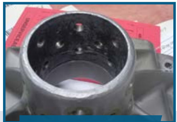
Cracked rudder torque tube coupling
