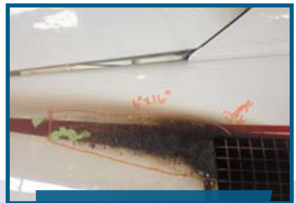
Evidence of auxiliary power unit distress on tailcone
