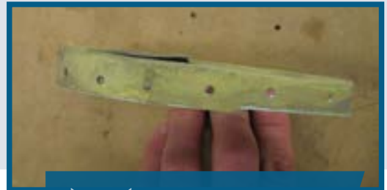
Top view of the cracked rib
