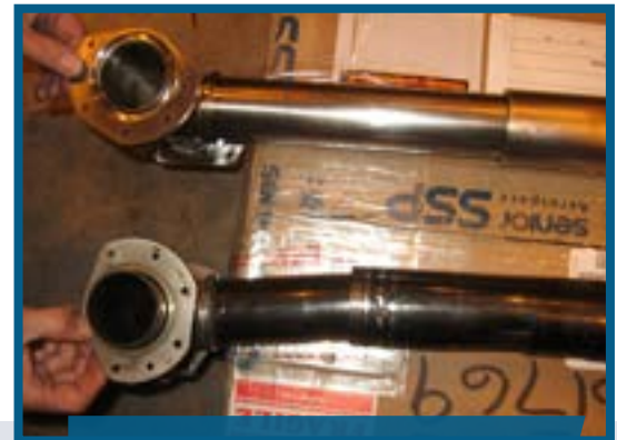
The bent telescopic anti-ice duct in comparison to a serviceable one
