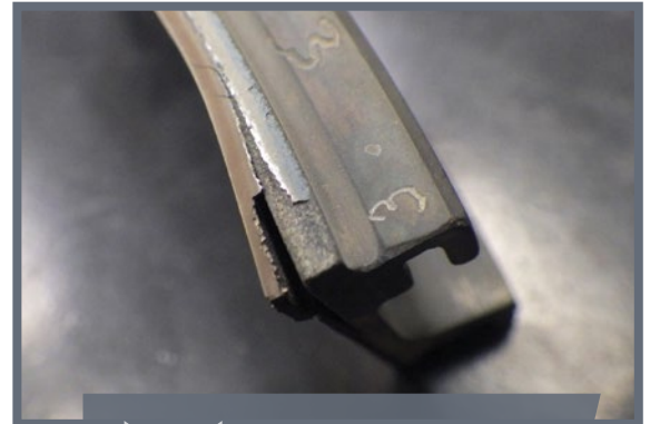
High pressure turbine shroud segment with evidence of delamination
