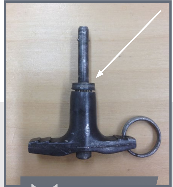
Cracked Release T Handle P/N 204-072-727-013
