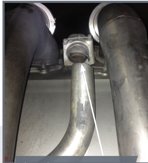
Missing engine cowl blow-out panel and failed anti-ice duct
