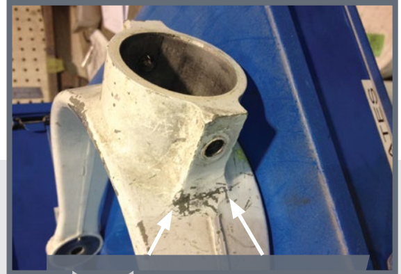
View of the cracked nose gear fork
