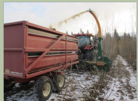
Figure 5. Willow harvest with modified sugar cane harvester
